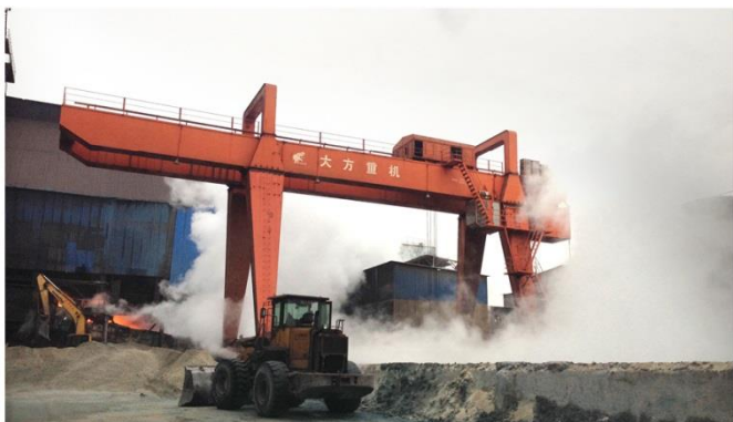
唐山海特钢集团室外干渣作业区使用的大方重机双梁龙门产品。 Double girder gantry crane made by DA Fang Heavy machinery co.,ltd used on outdoor dry slag operation area in Tangshan Donghai special steel group
