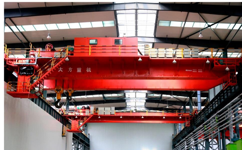
发往青岛德铸特钢集团的 125T 具备防摇摆和精确定位功能的冶金双梁起重机 metallurgy double girder crane with anti-sway and accurate positioning function used in Hebei steel group Tang steel high-strength auto-steel project
