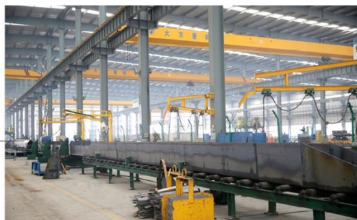
主梁组对 main girder assembly
