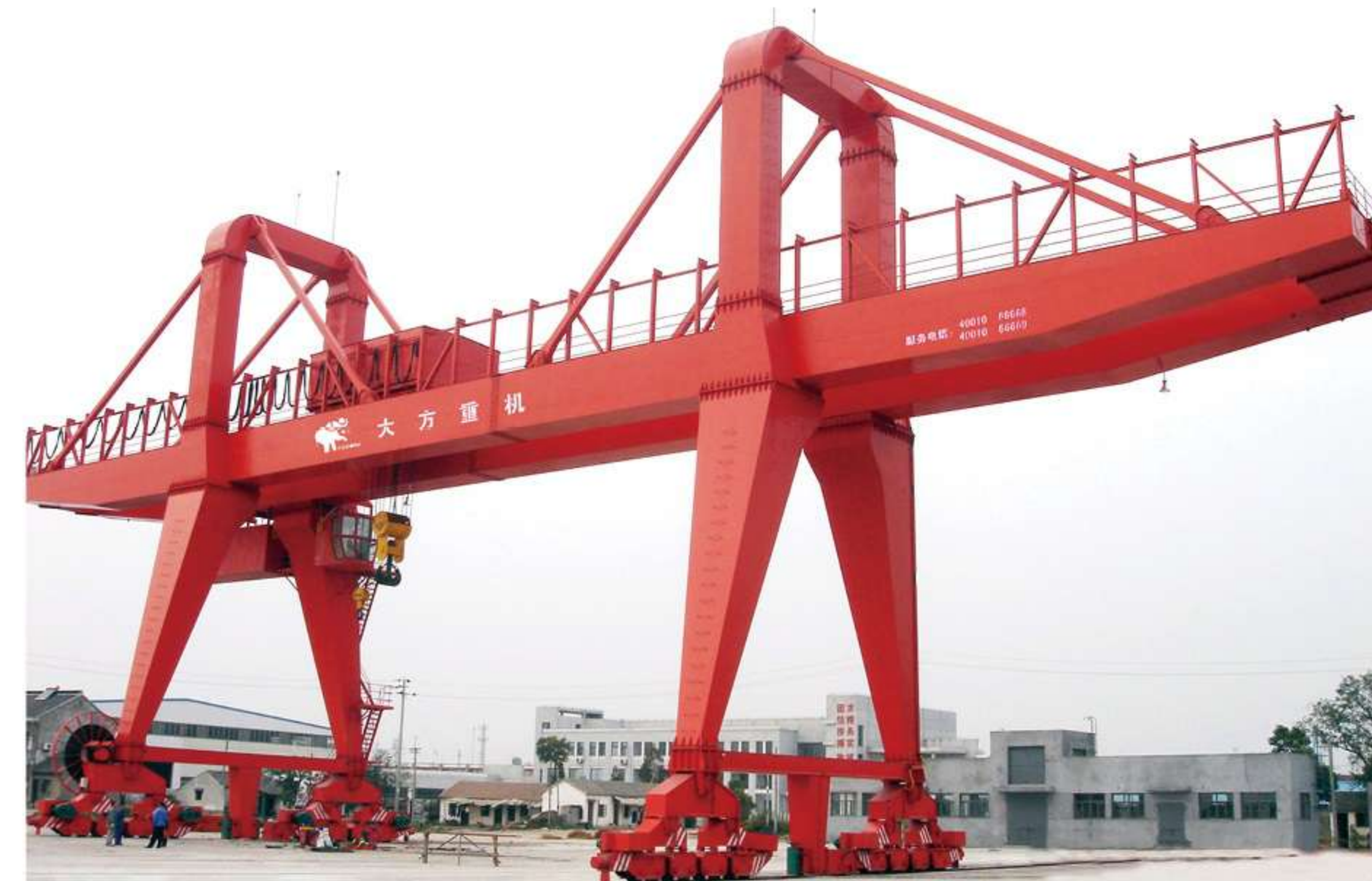
装卸桥 loading bridge
