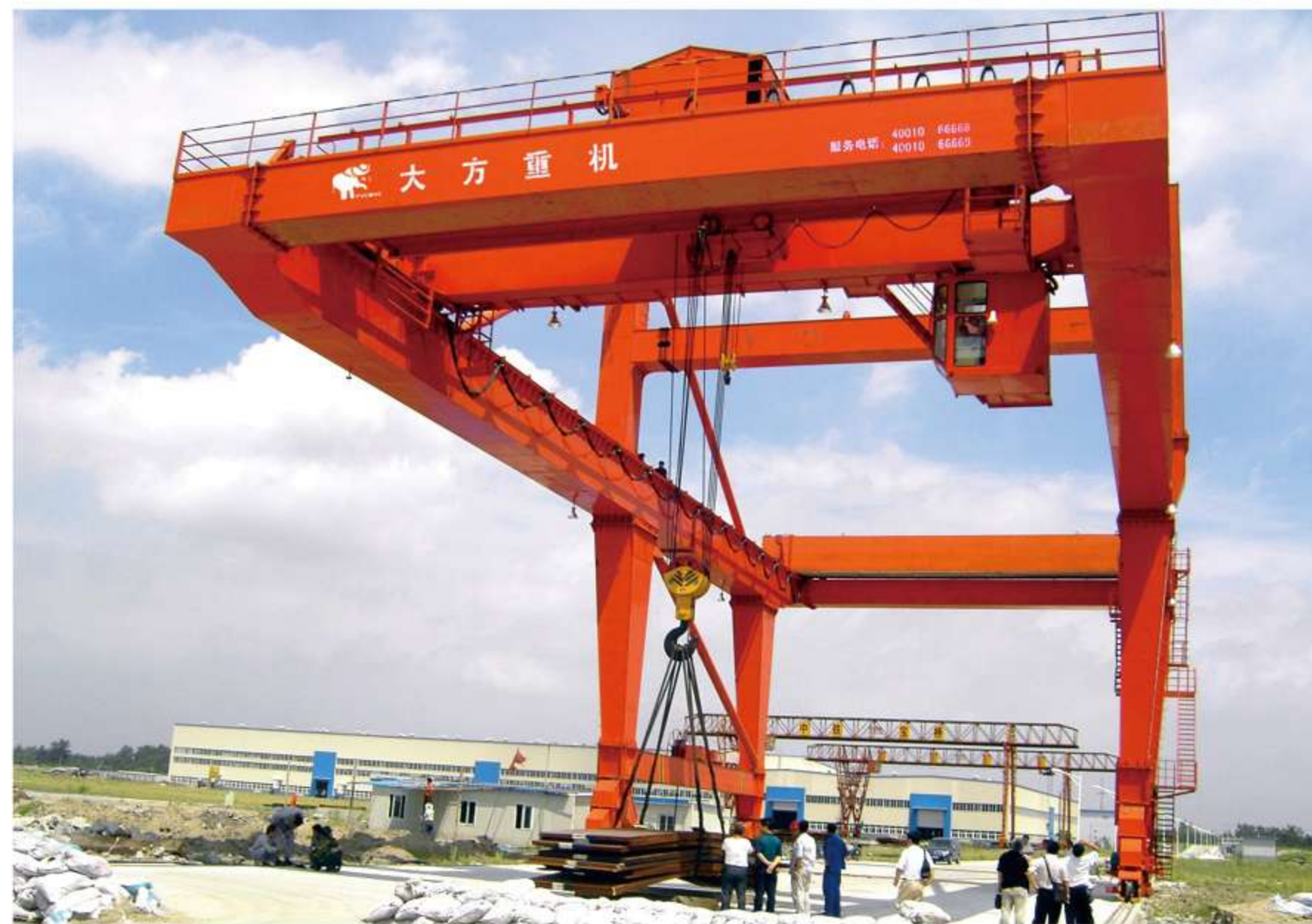
装卸桥 loading bridge
