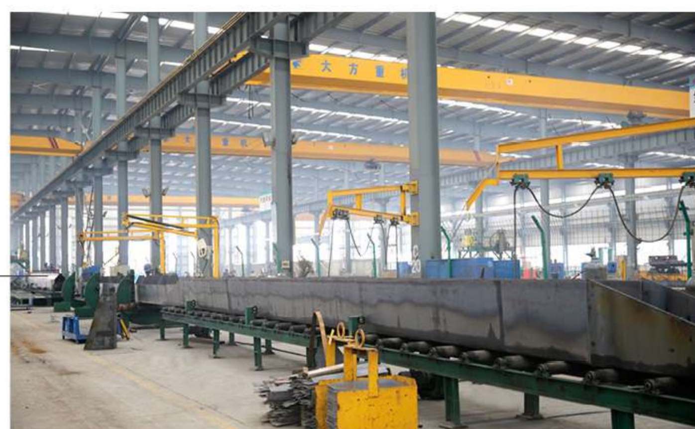
主梁组对 main girder assembly
