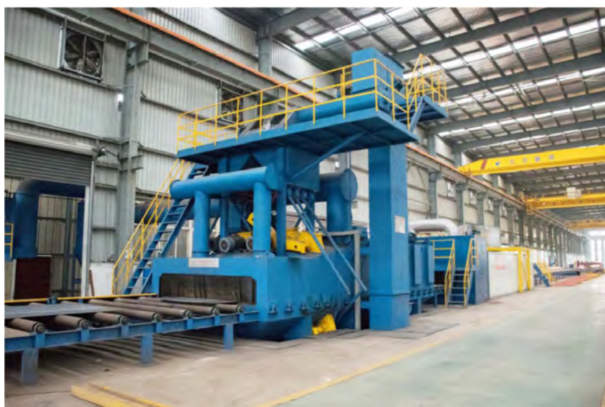
Shot Blasting Processing
